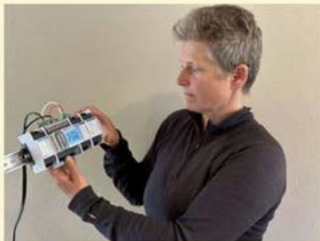
Sascha with a micro-PMU, a sensor used in smart grid technology.
