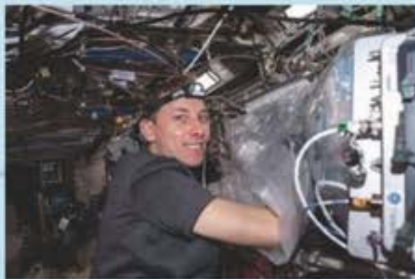
Woody Hoburg, astronaut on the International Space Station, changes the bio-ink on a 3D bio-printer that prints in micro-gravity.
